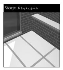
4.When all boards have been firmly placed and fixed ,the joints can then be taped using a water-proofing system. The material used for taping and sealing the joints should be suitable for exterior
