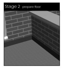
2.Prepare the existing floor ensuring all traces of grease and dust are removed. Place 5mm expansion strip to the perimeter to ensure an expansion joint is maintained between the wedge board and the wall. This joint will be sealed at a later stage with a suitable sealant.
